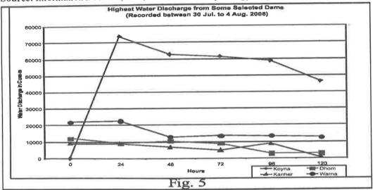
The discharge from the Koyna dam was one-lakh cusecs on July 30, 2006 and this trend continued for long time. Except major dams, minor dams had also higher discharge during flood period in both years. The Figure 4 and 5 shows the trend of water discharge from the Koyna, Warna, Dhom and Kanher dams (Table III and IV).
