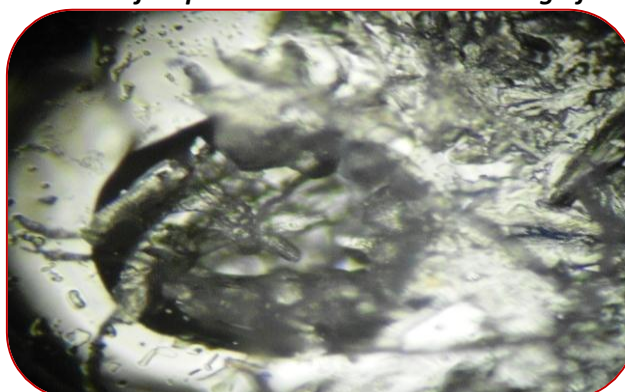
I-B. Typical photographs of 35% \text{Na}_2\text{O} content glass samples for various time of exposure in 10% NaOH at 20X magnification.
